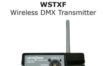
The WSTXF is a compact RF transmitter unit which transmits a USITT DMX-512 lighting control signal. It's input signal is received from a normal wired DMX system via a standard 5 pin male XLR connector. The WSTXF is supplied with a UL listed external power supply and an transmitting antenna.
