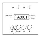
Press the MODE button to access receive (DMX) mode. An "A" in the display indicates receive mode. There will also be a small indicator illuminated on the top right side of the display next to the "Receive" text. In addition, if you've connected your DMX console to the pack, there will be a flashing indicator in the top left side of the display next to the "DMX Signal" text indicating that DMX signal is present.
