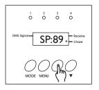
Tap the up ▲ or down ▼ buttons to set your desired chase speed. The range is from 01-99. The higher the value, the faster the chase speed.
