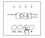
6. Press the up ▲ or down ▼ buttons to change between dimmer / switch modes. Once set, press the MENU button to confirm and advance to the following channel settings. Repeat these steps for all four channels. When complete, the DMX channel address setting will show in the display.
