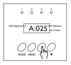
2. Tap the up ▲ or down ▼ buttons to set your desired DMX channel address setting. Pressing and holding the up or down buttons will change the values in the display quickly. This is useful when trying to achieve higher channel values.
