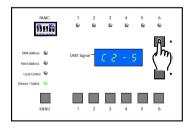
(2) Press the UP/ Down button to change the current setting. d="Dim"/s="Switch"
