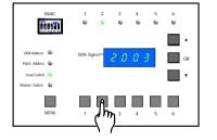
(1) Select the channel that you wish to manually control by selecting from buttons 1-6. Only one channel can be selected at a time.
