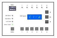
Press the MENU button until the "Dimmer/Switch" LED illuminates. The display will read either " creat " or " creat" depending on the current setting. The "C" indicates "Channel". The number that follows is the pack's channel number. The "d" indicates "Dim" and "S" indicates "Switch". In the example to the left, it shows channel 1 is currently set to dim.
