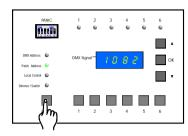
Press the MENU button until the Patch Address LED illuminates. The display will show you the current patch setting for channel 1. For example, if channel 1 was set to DMX channel 82, the display would read the following: TO GO . The number 1 in the display indicates channel 1 of the pack. The next three digits indicate the current DMX address for the selected channel.
