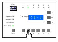
(1) Select the channel that you wish to assign by selecting from buttons 1-6. Only one channel can be assigned at a time.
