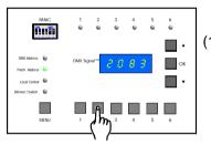
(1) Select a channel button that you want to address. Use the UP/DOWN button to adjust the channel setting. The address can be set anywhere between 001-512.
