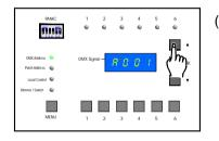
(1) This function is used when setting the starting DMX address channel for the pack. Use the UP/DOWN buttons to adjust to a desired setting. The selected DMX channel will be the DMX starting address for the pack. A total of six DMX channels will be occupied by the DP-640B in sequence, starting with the set channel.
