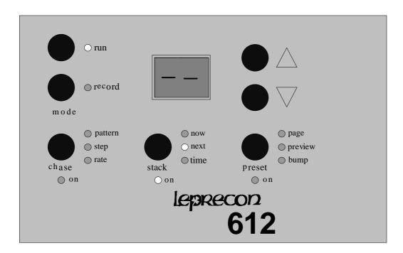
When 'next' has been set to the blank scene, press the 'stack' menu button again to light the 'time' Led. Enter the time desired as the default time for all scenes.
