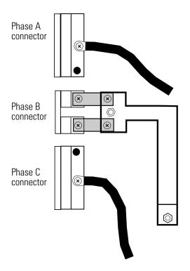
Phase connectors wired for three phase operation
