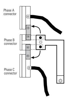
Phase connectors wired for single phase operation
