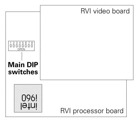
If the settings get changed and you need to restore them, find the switches at location **S4** and adjust the settings as listed below. The RVI checks DIP switch settings when the unit is turned on. You must restart the unit for the new settings to take effect.
