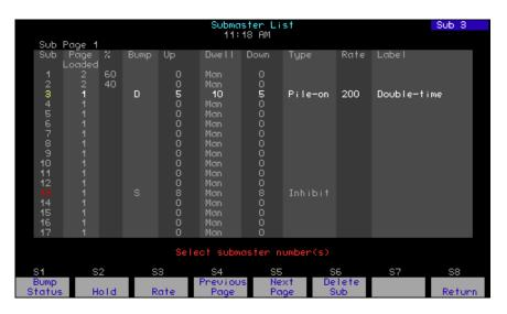
The first 17 submasters are shown initially in the Submaster List. Page through the rest of the submasters using the [S5], **Next Page** and [S4], **Previous Page**, keys.
