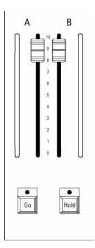
Each fader slider has a strip of LEDs next to it. When running a timed crossfade cue, the lit LEDs indicate the progress of the cue. This is displayed as a percentage. For example, when the LEDs are at **5**, 50 percent of the cue has run.
