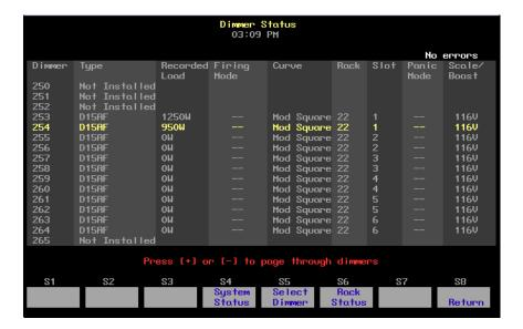
Up to 16 dimmers are shown in the display at once. If a dimmer has an error condition, the entire dimmer row is highlighted in yellow (ordinarily the line is in gray). Dimmer errors are also identified in the About Dimmer display. See About Dimmer with ETCLink, page 52.
