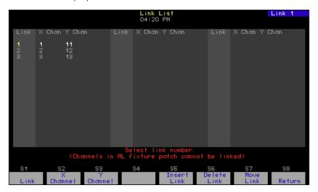
When two or more channels are used together, such as the color and intensity channels for a color scroller, the Link List allows you to determine which of the wheels will control each channel. When you select a channel, it is placed under the control of one of the wheels and all channels linked to it are also selected and placed under control of the other wheel.
