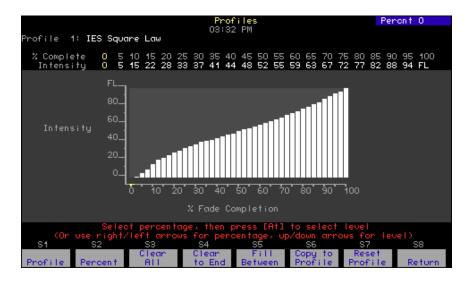
The Profiles display contains a bar chart, with the total time for completion of the fade broken down into 40 equally spaced bars. The height of each bar represents the percentage of the full fade level defined as intensity. Twenty of these bars are editable for intensity and are called fade points. In between the 20 editable fade points are the remaining 20 bars, and these indicate the calculated intensity levels between fade points.
