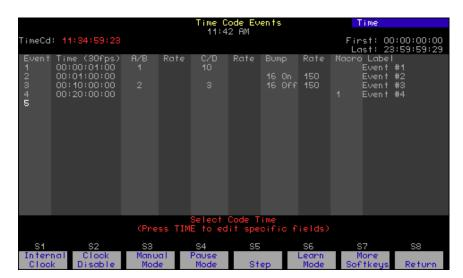
For all procedures in this chapter involving programming in the Time Code Events display, press [Setup] [1][3], **Time Code Events**, [Enter] [Enter] to go to that display. In the display:
