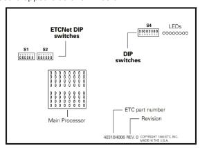
When installing ETCNet, Full Tracking Backup or SMPTE for an earlier model console, adjust the processor board's DIP switches according to the information below.
