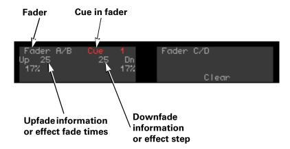
The fader status display provides information about the cues loaded to the console's faders, including fade times and rates. The left window monitors the A/B fader; the right window monitors the C/D fader. The display counts down wait times for cues and indicates which step is running when an effect is active.
