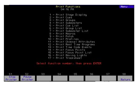
You may pause the current printing job or cancel it at any time while printing. To stop the printer temporarily while it is printing, press [S2], **Pause Printer**. The printer prints a few more lines, then stops and waits. Press [S2] again to resume printing. To cancel a print job, press [S1], **Stop Printer**. The printer prints a few more lines, then stops.
