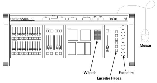
For each page, attributes are assigned by default to encoders, wheels and to the two axes of a pointing device. You can change the default assignments to suit your needs or preferences, such as if your console is not equipped with a pointing device.
