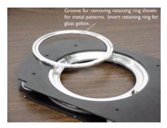
To remove the ring, place a small tool in the groove provided and pry the ring loose. When replacing the ring, align the small groove adjacent to one of the spring clips for easier removal.
