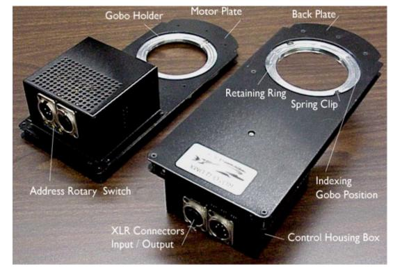
The rear gobo position is the indexable position. The pattern to be indexed should be placed in this rear gobo holder, i.e. closest to the lamp. This gobo holder is on the opposite side from the control-housing box.
