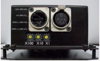
Some scroller power supplies have +24V DC on pin #1 rather than on pin #4. The polarity of the pins should be carefully examined. Several manufacturers produce individual power units with two different configurations, so brand identification can be misleading.
